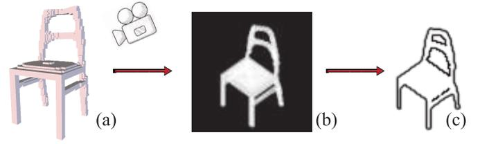
Fig. 4. Illustration of training sketch generation. Starting from a 3D shape and a view angle in (a), we first project the shape to an attenuation image in (b), and then extract a sketch from the attenuation image in (c) using the Moore-Neighbor tracing algorithm.
